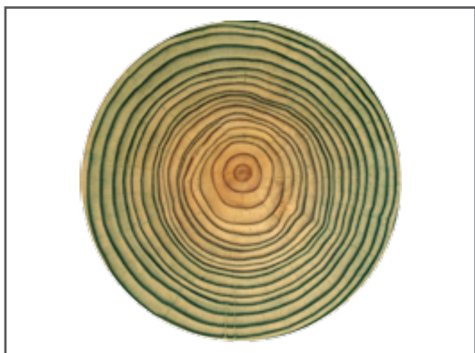
Impregnation round utility poles
